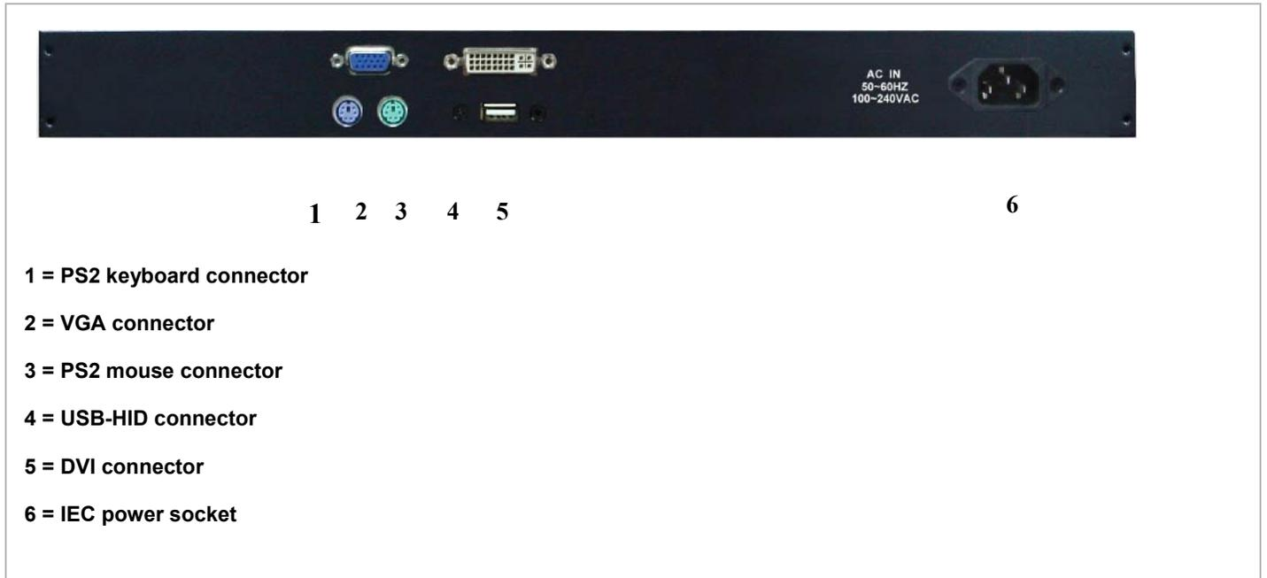
Figure 2. RackView rear panel connector layout
