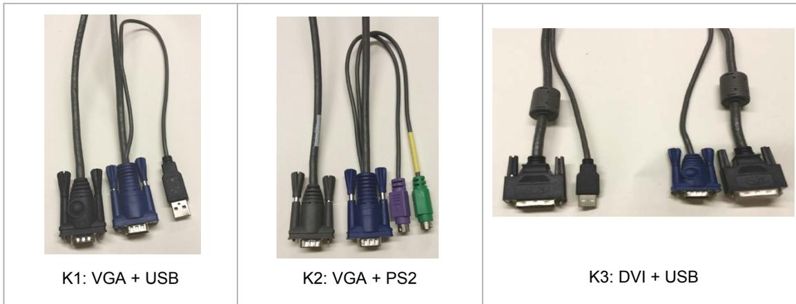
Figure 6. RackView device interface cables
