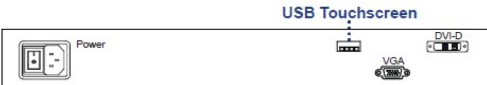
Back panel of Rackview LCD Touchscreen Monitor, showing the location of the connectors.
