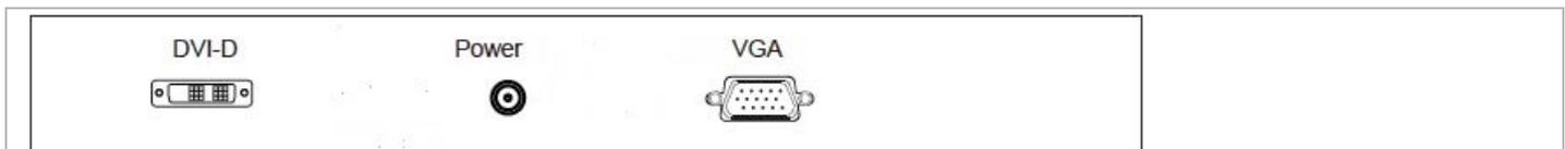
RackView LCD Panel - rear panel connector layout for the standard interface
