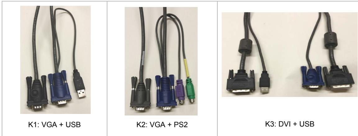
Figure 6. RackView device interface cables
