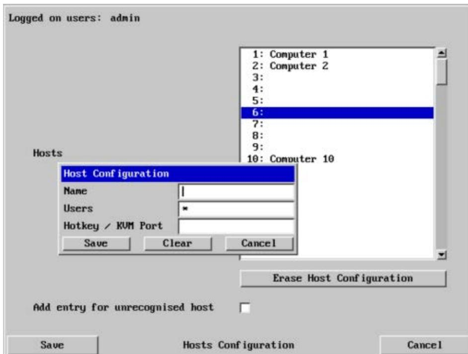
Figure 20. Host Configuration window
