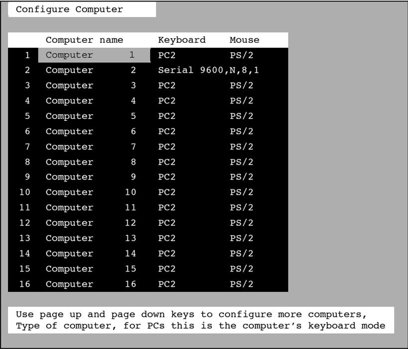
With the CPU port configured for serial support and the appropriate serial cable connected, the KVM station can access the connected serial device the same way you would access it using a computer terminal.
