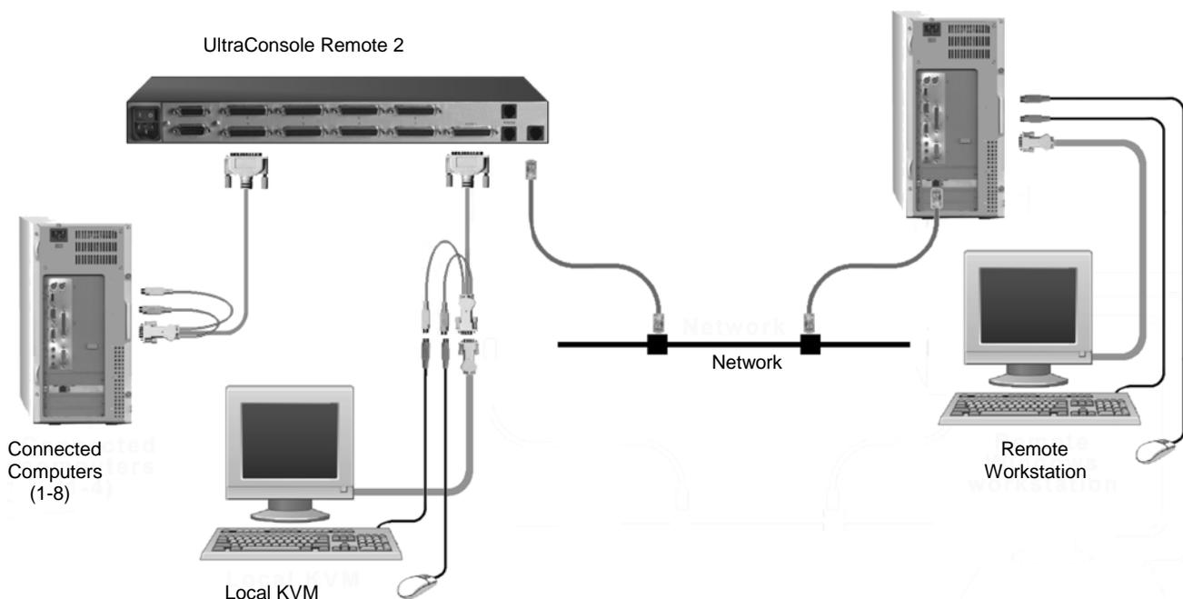
Figure 1. Typical Single Unit Application
