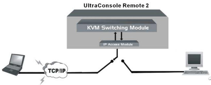
The UltraConsole Remote 2 consists of an IP input module and a KVM switch module. The IP input module controls unit access, locally and remotely, and access security. The KVM switch module controls the port switching and has its own unique OSD that can be configured with appearances, port settings, additional security, and other parameters.
