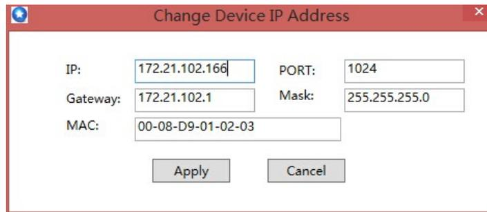
Figure 17. Change Device IP Address Screen
