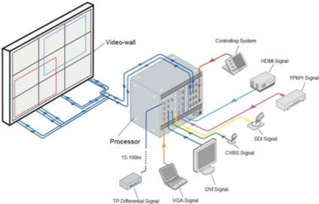
Figure 10. System Diagram of UltraVista Pro
