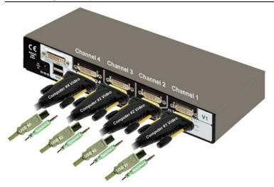
Up to 4 single head computers can be connected to the Vista DVI Plus unit. (8 single head computers on the 1 x 8 model)
