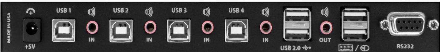
Figure 2. KM-4USB- III Rear Panel
