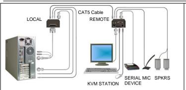
Depending on your model, cables and rear panel connectors will vary. A KVM station can be connected to models with local access.
