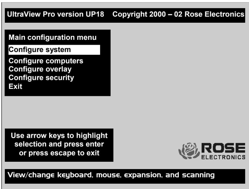
To navigate through the menu system, use the arrow keys to select the configuration menu needed and press [Enter]. When you press [Enter] that menu will display, an input box will display for a new value, or a list of supported choices will display. Enter or select the information needed and press [Enter]. To return to the previous page or abort an input, press the [Esc] key.
