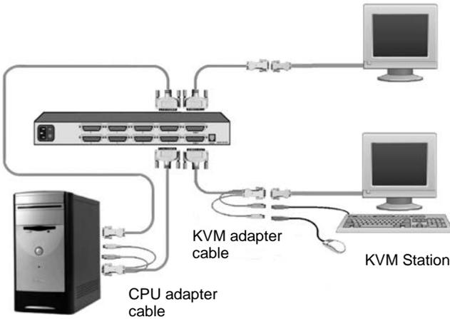
1. Connect a KVM station to the KVM, DB25F connector using the appropriate KVM adapter cable.
