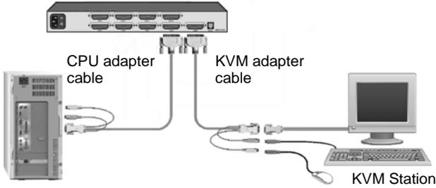
1. Connect a KVM station to the KVM, DB25F connector using the appropriate KVM adapter cable.
