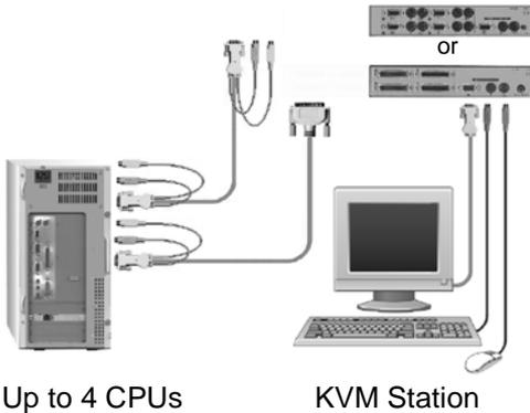
1. Connect the KVM station's keyboard, monitor, and mouse cables to the corresponding Vista KVL switch ports.
